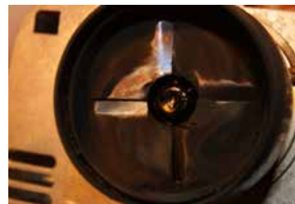
Fig. 8 View of the damaged fuel head in the burner
