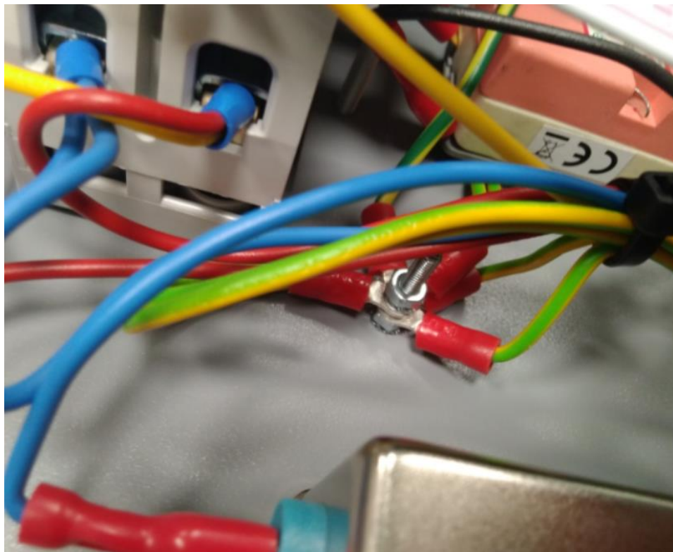
Earthing terminal (to be added symbol)
