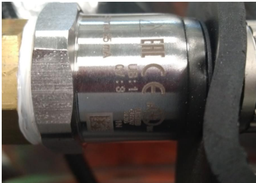
Pressure transducer markings
